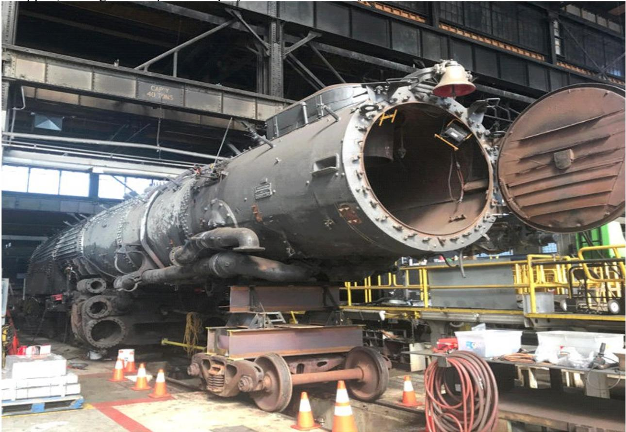
**UP 4014 is seen disassembled at the railroad's restoration facility in Cheyenne**
